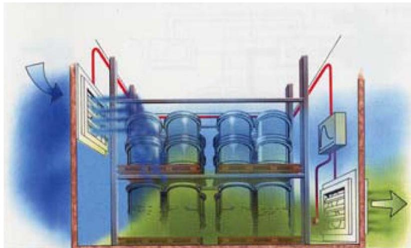
Example of proper ventilation of a contained room with heavier than air mixtures.
